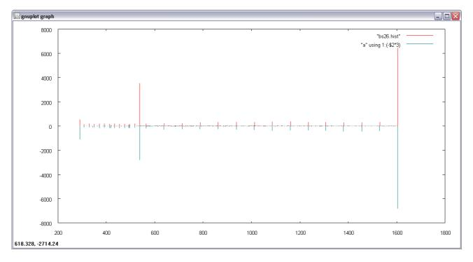
Here the +ve lines from zero upwards are the actual histogram of hit frequencies observed. The -ve lines are as predicted by my model. The model is, as can be seen, not entirely accurate.
